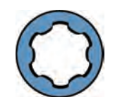
TORX PLUS® drive bit in TORX PLUS® recess
