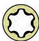
TORX® drive bit in TORX PLUS® recess
