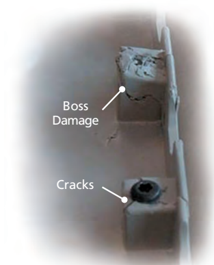
Fig.7. Assemblies with self-tapping screws on a polyester piece with 30% fiberglass cause cause boss cracking.
