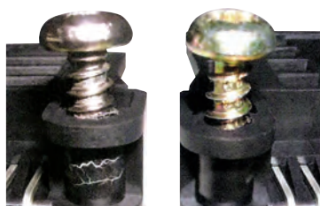
Fig.6. The reduction of radial tension during thread forming of REMFORM® screws helps to prevent boss bursting.
